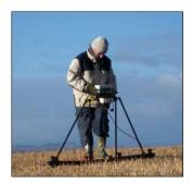
array of mobile and remote electrodes maintained at a distance of about 20m.
